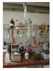
account. The latter cannot be determined or estimated theoretically, but require the possibility of a visual evaluation of the evaporation process. This can best be implemented in glass plants from COROSYS, which can be individually assembled on the basis of a modular system.
